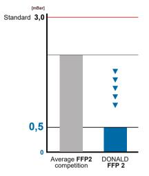
Half-mask that has one of the lowest breathing levels on the market. Air flow of 95l/min is the approximate value of breath when working in heavier environments
